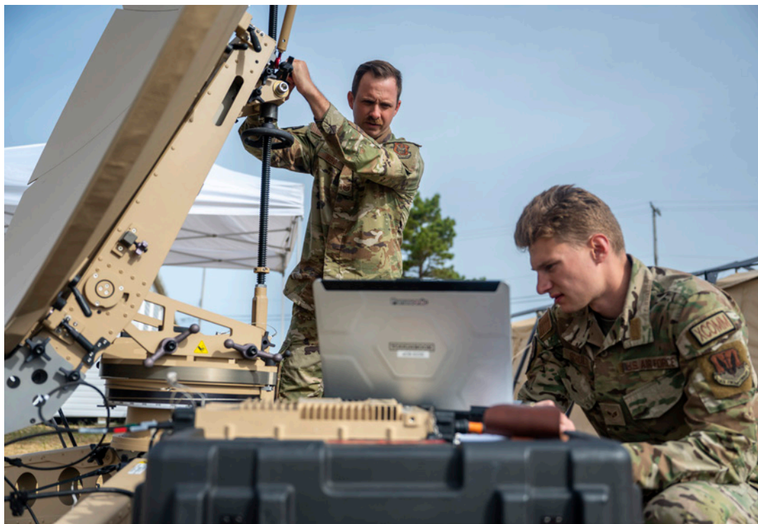
U.S. Air Force Tech. Sgt. Joshua Werho, 55th Combat Communication Squadron radio frequency transmission systems technician, and Senior Airman Jesse Severns, 35th CBCS cyber security technician, check operations on a Ranger 2400 Flyaway Multi-Band Terminal during EXERCISE AGILE BLIZZARD-UNIFIED VISION 2023 near Comox, British Columbia, Canada, June 19, 2023. The satellite dish allows for quick setup satellite communications which is necessary when operating in a semi-austere location where communications are limited. (U.S. Air Force photo by Tech. Sgt. Betty R. Chevalier)
