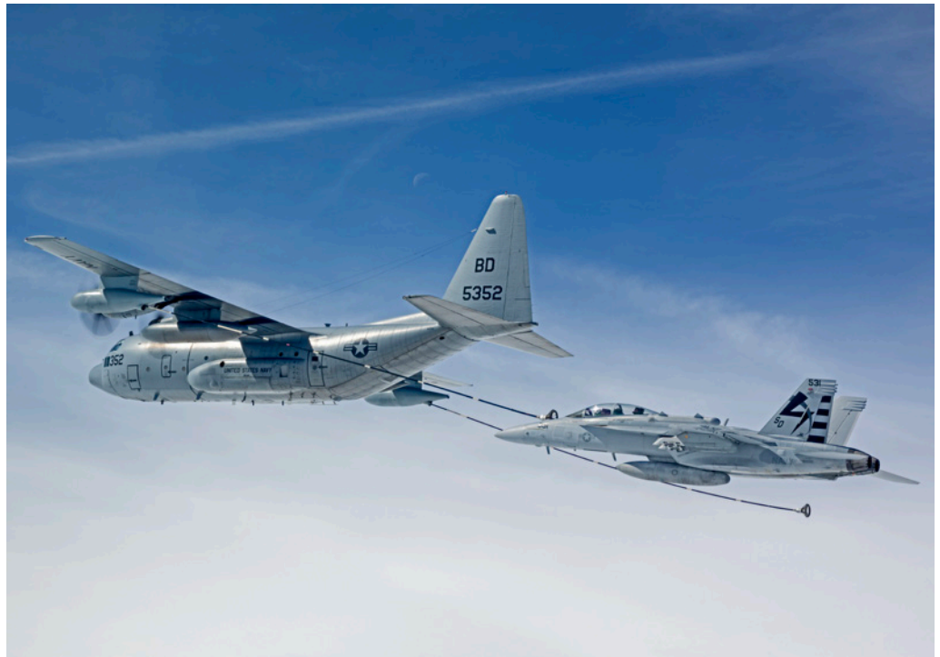
A Fleet Logistics Support Squadron 64 (VR-64) KC-130T Hercules conducts dual-hose aerial refueling testing at Naval Air Station Patuxent River. (U.S. Navy photo)
